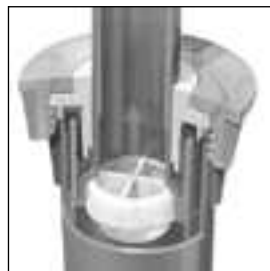
Seal grips riser at top and bottom—eliminating wasteful flow-by
